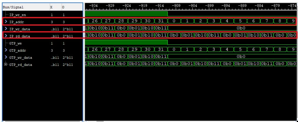
图 2.3-5 Distributed Single Port RAM 读操作测试 (IP)
