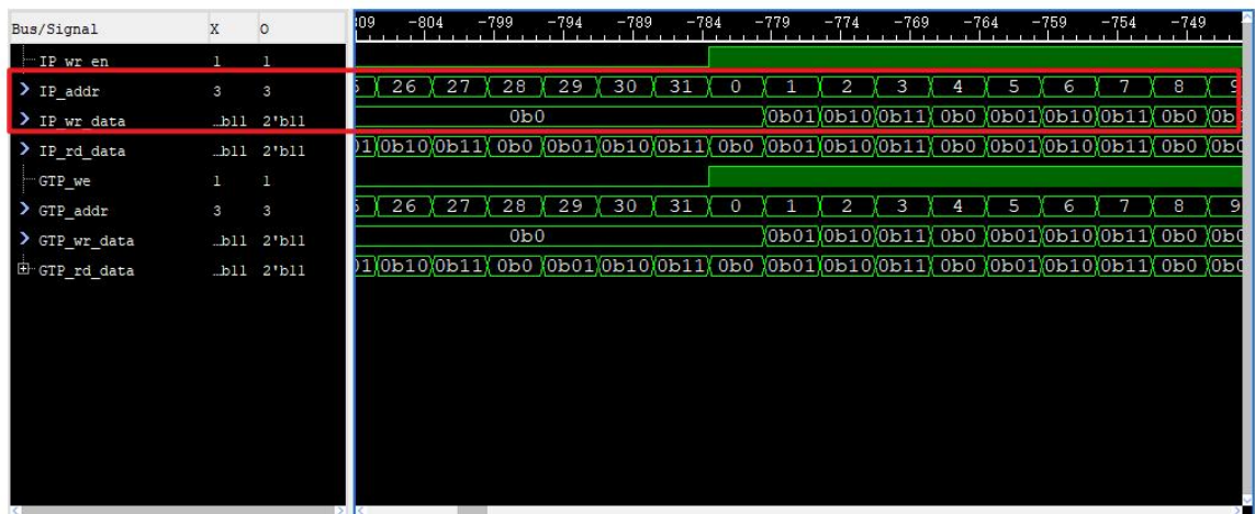
图 2.3-3 Distributed Single Port RAM 写操作测试 (IP)
